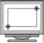
*Calibration* aligns the touchscreen with the underlying video. Specifically, calibration defines the dimensions of the image area of the touchscreen, determines the edges of the screen's image, and locates the center of the touchscreen. You must calibrate the touchscreen and test the calibration to ensure the successful operation of the touchscreen.
